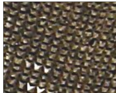
Trizact EA™ manufactured for uniform cutting
